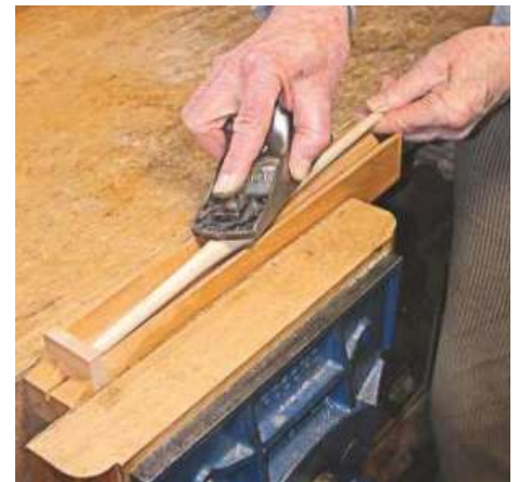
▲ Pic. 10 Making final touches to the flat with a block plane
